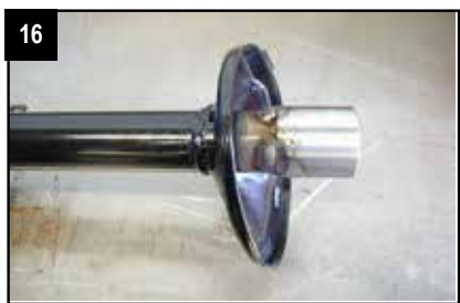
16. WELDED ADAPTOR SHOWN.
