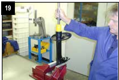
19. PLACE THE CARTRIDGE ALL THE WAY INTO THE STRUT THEN LIFT OUT TO CHECK OIL LEVEL.
