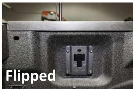
1. With the bed Cleat reinstalled we can slip the Compressor assembly into the cleat. Make sure the T Nut (03-525-1) has enough room to slide into the cleat.
