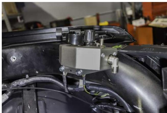
6. With the ADS Controller in Place we can run the preassembled 3/8" Lines. The Long leg of the 3/8" line will run along the Firewall to the passenger side fender well. The 32" line will run down the Driver side Fender well and the 26.7" Line will run up to the ADS Controller. The "T" connector should land on the driver side of the Master Cylinder Assembly.
