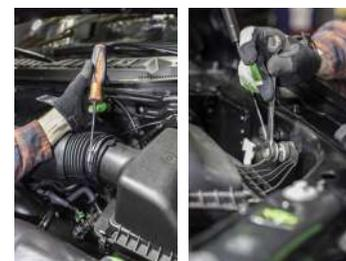
4. Remove the entire air box Assembly. It will lift out with a little wiggle. It has 2 rubber grommets that hold the bottom in place.
