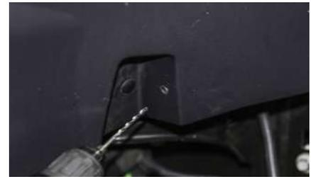
8. For the Front you will want to locate the small recess near the bottom of the fender well near the cab. It has a small Flat Surface that faces towards the outside of the vehicle. You will need to drill a 5/16” hole to mount the Schrader valve. Mount the Schrader valve on the Driver and Passenger side with supplied washers and nut.
