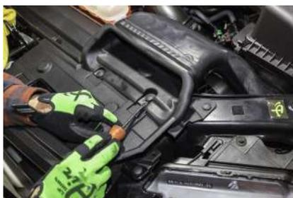
3. Loosen the Clamp for the Air filter box and support bolt on the inner fender to remove complete Air box assembly.
