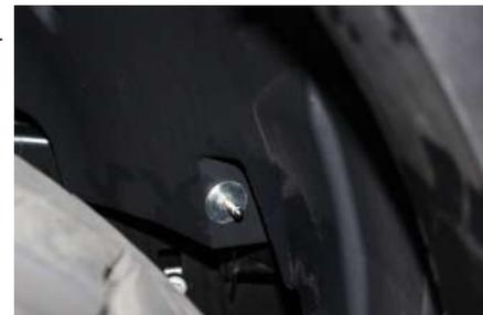
9. For the Rear you will locate the smooth area of the fender well in front of the tire (Front Side of the Fender Well) just inside of the fender flare. Approximately 10” up from the bottom of the fender. Drill a 5/16” hole to mount the Schrader Valve. Mount the Schrader valve on the Driver and Passenger side with supplied washers and nut.
