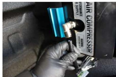
9. We recommend using zip ties to loom the Power cables and High Temp 3/8 Airline together.
