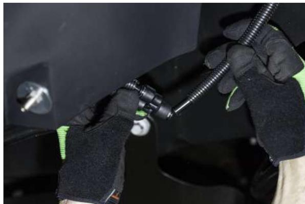
11. With the lines secured under the vehicle we can connect the Main Feed Line from the compressor and the  $\frac{3}{8}$ " distribution line to the ADS Controller. The Compressor feed Line will connect on the left side of the ADS (Closest to the Schrader Valve on ADS) and the Distribution line will connect on the right Side (Closest to the Bleed Valve on ADS)
