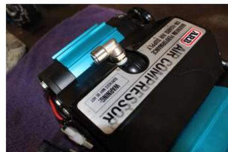
5. Locate the wiring harness for the ARB Compressor and Harness Extension. Connect the wires together to create one long loom.
