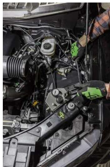
12. With the completion of the ADS System we can re install the Air box assembly. It will be a snug fit with the ADS Controller in place. We recommend installing the lower half of the air box first leaving the inner fender bolt out until the air box lid and intake are securely in place. This allows the air box to wiggle for extra clearance. Once the air box, lid and intake are in place install the inner fender bolt to secure the air box assembly.
