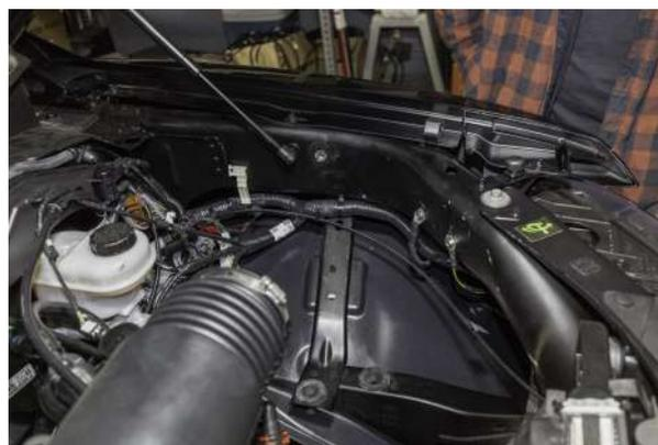
5. With the Air Box removed there will be 2 Bolts on the core support with ground wires connected. Remove the Bolts. Install the ADS Controller with the OEM bolts. **\*\*\* Be sure to re connect the ground wires when installing the ADS Controller to the core support\*\*\***
