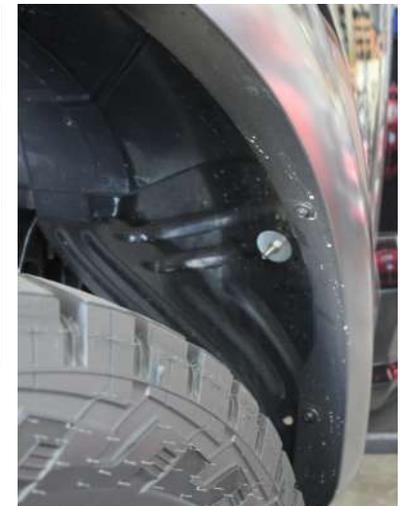
10. Once the Schrader valves are secured in the fender wells the pre assembly is complete. The next step is to mount the ADS Controller in the engine compartment.
