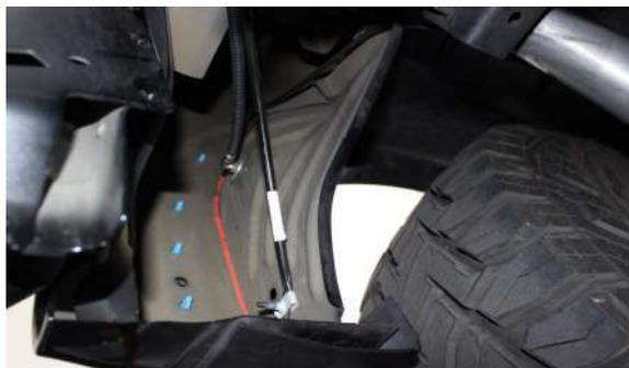
10. Once the Front and Rear and Rear Schrader Valves have been connected to the  $\frac{1}{4}$ " lines the  $\frac{3}{8}$ " lines located at the front fender well can be connected to the "Y" connectors. All of the connections have been completed under the vehicle. Be sure to secure all air lines to prevent damage.
