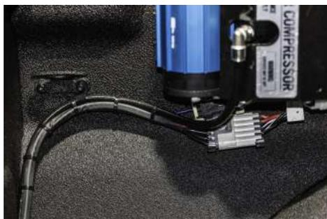
10. With the Compressor assembly and Lines bundled in the bed we can move on to routing the power cables. Feed them along the frame rail above the Body Mounts.
