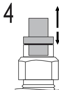
**Removal Tip:** Use a small open-ended wrench to push the collar down .
