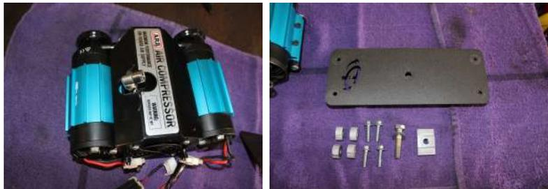
2. Install T Nut (03-525-1) and 3/8-24 Bolt with washer into ARB Compressor Bed Mount (03-525). Leave Bolt and Nut loose to allow room to slide into bed Cleat with compressor assembly.
