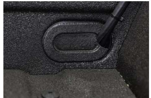
4. Notch the Dust Cover to allow the Power Cables and Feed Line for the compressor to pass through the Dust Cover.
