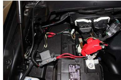
7. The 3/8 " Crossover line on the Firewall should run in parallel to the 3/8" feed line from the ARB compressor.
