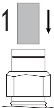
Push Air Line Tube into Air Fitting as far as possible.
