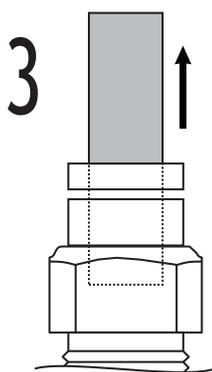
To remove, push down collar and gently pull Air Line Tube away.
