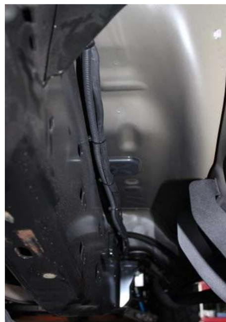
11. Once they reach the Passenger Fender well they will run up the back side of the fender to the engine compartment near the battery and ECU.
