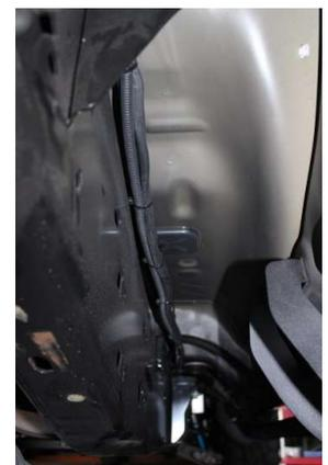
9. The Short Leg of the 1/4" line will connect to the Front Schrader valve. The long leg will connect to the Rear Schrader Valve.
