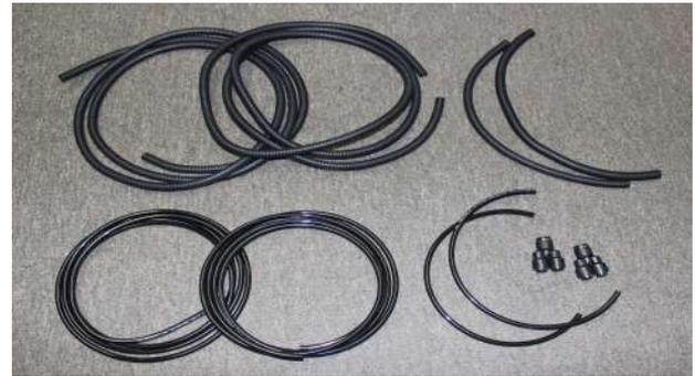
6. The ¼ inch lines will be installed into the parallel ports on the “Y” Connector. 1 Long and 1 Short per “Y” connector. With the ¼” lines installed the corresponding split loom can be installed on the lines. Once complete they can be set aside for installation.
