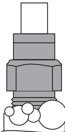
Tighten Air Fitting one turn or until leak stops.
