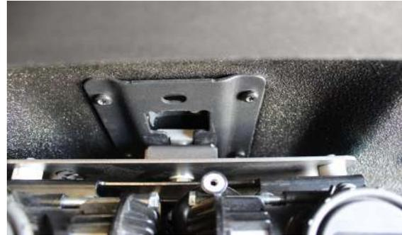
2. Tighten the 3/8 bolt for the Compressor Mount. It may be necessary to slightly rotate the compressor assembly to fit the wrench under the bed rail. The compressor should be level to the bed rail when fully tightened.
