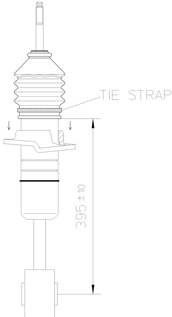
5. Reinstall coil spring, all original upper mount parts and upper spring seat in their original positions.
